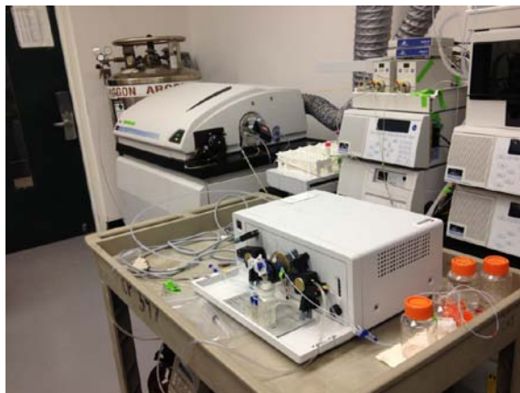
Figure 1. Coupling of a Flow Injection System (FIAS 400) to ICP-MS for analyzing mercury isotopes
