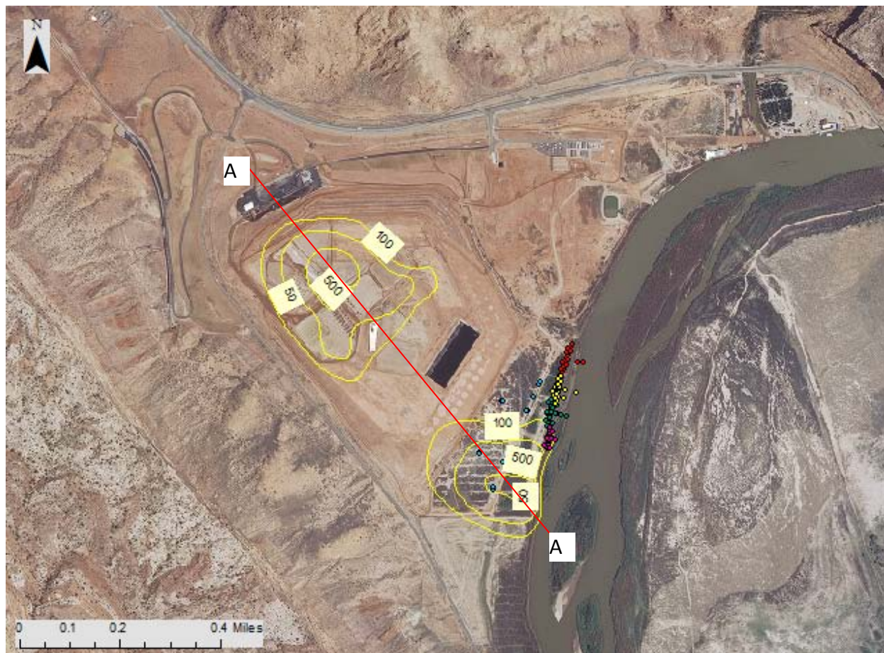
Figure 31 Ammonia (total as N) Concentrations Interpolated at 150 ft Below the Surface of the Ground Water (Section A-A is on the next figure)
