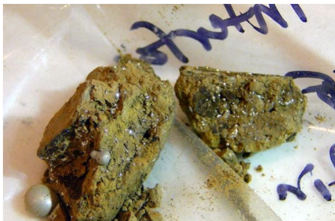
Figure 3. Mercury present in sub-surface soil samples from Oak Ridge (Applied Research Initiative, Oak Ridge National Laboratory, 2013).
