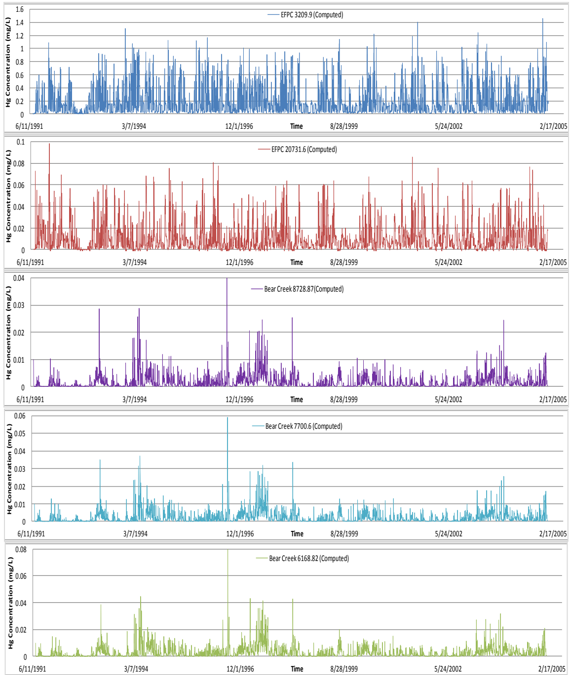
Figure 31. Computed mercury concentrations downstream EFPC and BC for various model nodes (EFPC 3209.9, EFPC 20731.6, BC 20731.6, BC 8728.87, BC 7700.06, and BC 6168.82).
