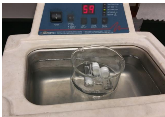
Figure 17. TEM suspensions undergoing sonication to disperse solids
