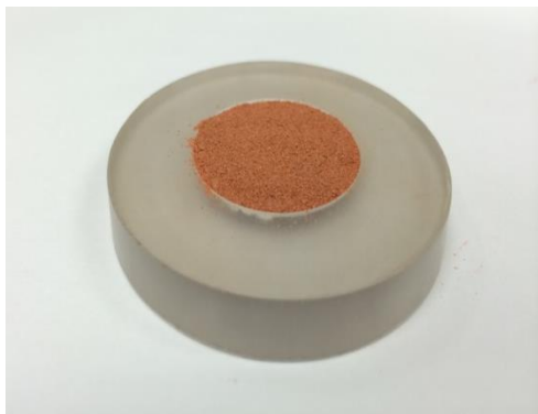
Figure 72. Amorphous sample holder with F-Area sediment to be placed into XRD instrument.
