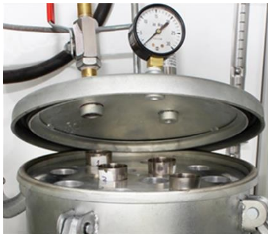
Figure 1. Isopiestic chamber to conduct solubility experiments; aluminum block with holes to hold nickel crucibles.
