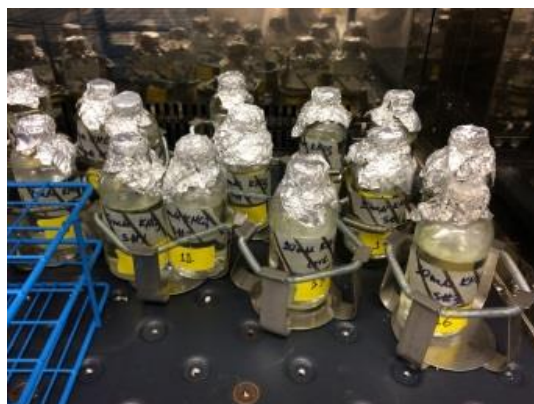
Figure 25. Experimental bottles placed in incubator-shaker at 20°C for autunite dissolution studies.
