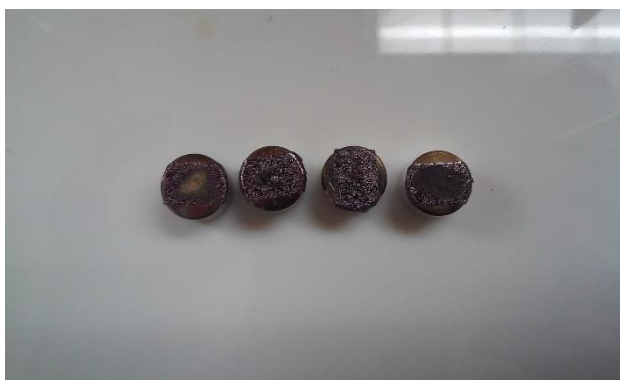
Figure 99. Samples coated with Gold/Palladium for SEM/EDS analysis
