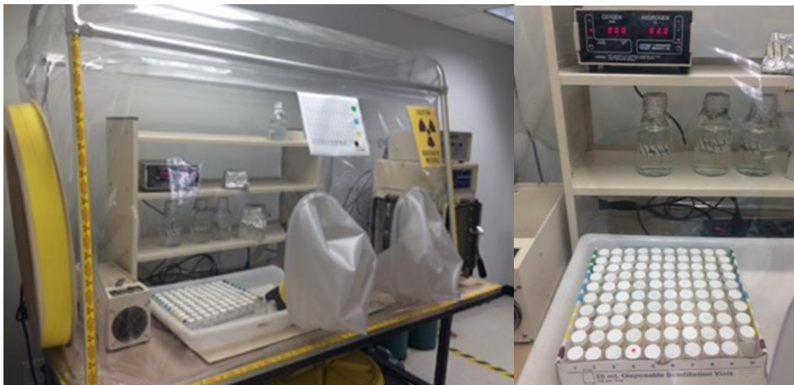
Figure 37. Sacrificial vials inside the anaerobic glove box, prepared to conduct the autunite biodissolution experiment.
