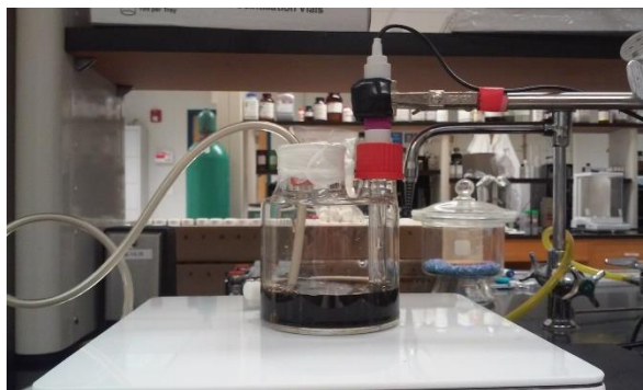
Figure 100. Setup for the Potentiometric Titration
