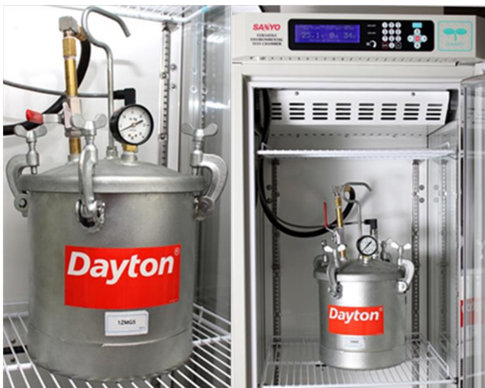
Figure 3. Isopiestic chamber to conduct solubility experiments connected to the acquisition system.
