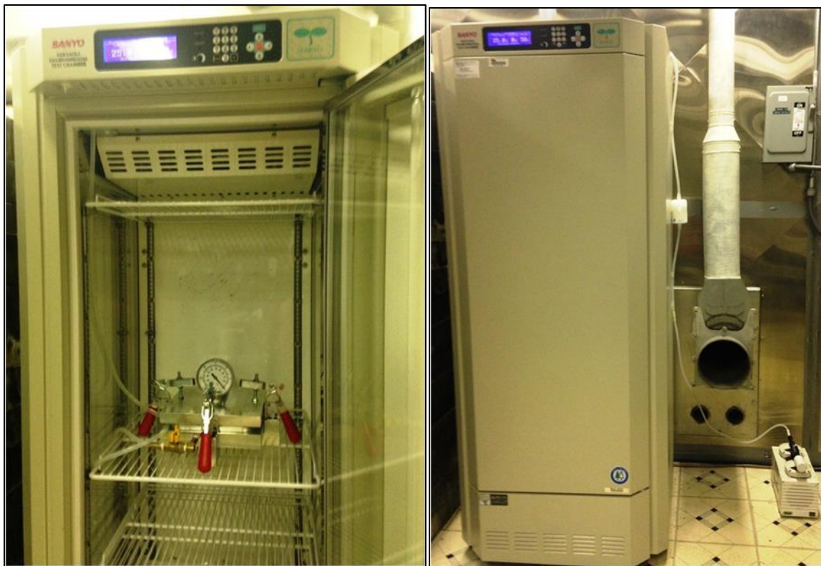
Figure 14. A new isopiestic chamber set up in the FIU-ARC radiation laboratory.
