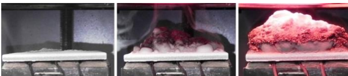
Figure 9. Intumescent coating reacting to flame / heat source. (Source: One Stop Shop in Structural Fire Engineering, Professor Colin Bailey, University of Manchester).
