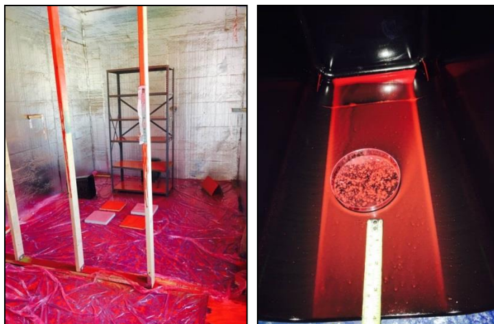
Figure 8. Red-tinted FX2 agent covers all horizontal surfaces in 10'x15'x10' hot cell mockup after fogging (left). Fogged challenge sample located inside apparatus facing away from foggers (right).
