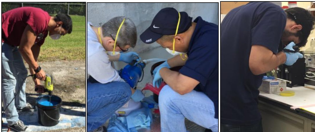
Figure 6. Mixing FX2 (left), filling fogger (middle), photographing sample for ImageJ (right).
