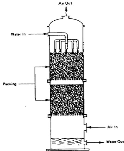
**Figure 2. Schematic diagram of a countercurrent air stripper used in the M1 air stripper.**
