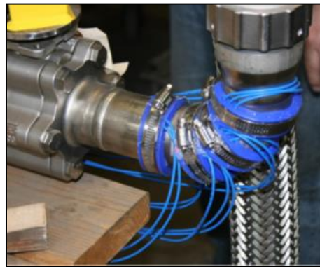
Figure 3. Installed Pipe Wrap™ system on a 2” diameter pipe [1].
