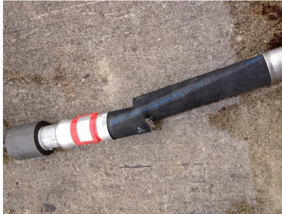
Figure 5. Failed hose specimen H-00-2.
