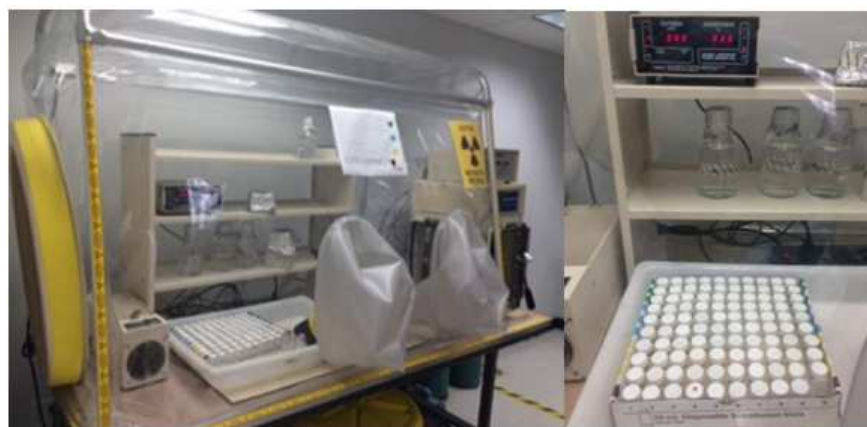
Figure 3. Sacrificial vials inside the anaerobic glove box, prepared to conduct the autunite biodissolution experiment.
