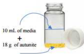
Figure 1. 20-mL glass scintillation vial prepared with media amended with \text{KHCO}_3 and autunite mineral.
