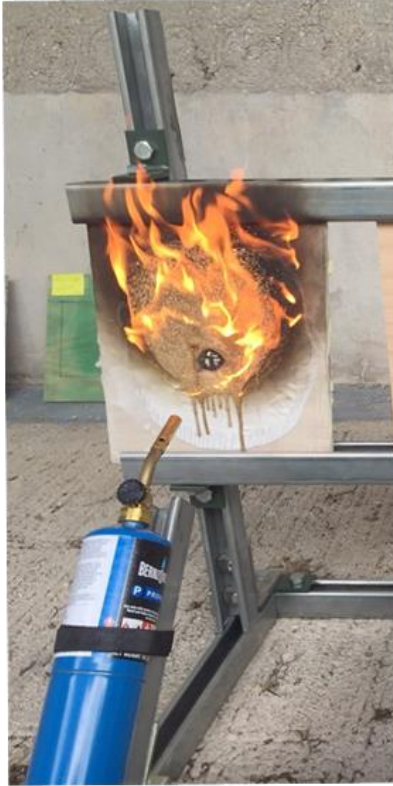
Figure 8. Fixative “B” burning off a red oak substrate test coupon.
