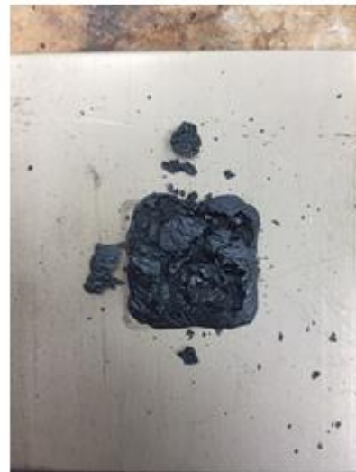
Significant mass loss, discoloration, desiccation, cracking, and flaking. Slightest abrasion with fixative resulted in total flaking. (800 degrees)
