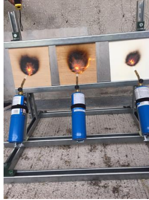
Figure 4. Open flame testing of fixative-only test coupons on red oak substrate.
