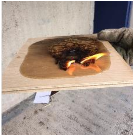
Figure 9. Fixative “A” continuing to burn after removal of flame source.
