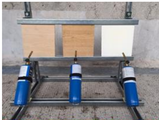
Figure 3. Open flame testing apparatus with 3 red oak test coupons.
