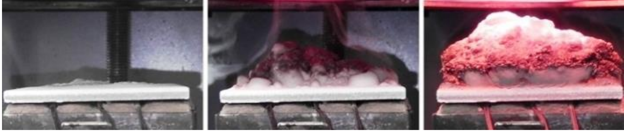
Figure 1. Intumescent coating reacting to flame/heat source.
