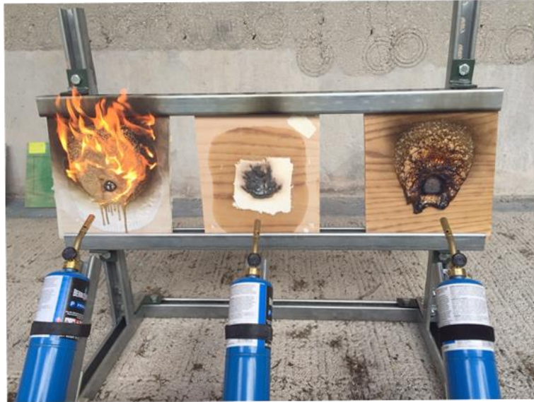
Figure 10. Demonstration of protection provided against flame when layered.
