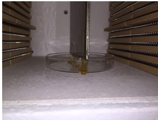
Figure 5. Fixative "A" on steel test coupon after exposure to 400°F in muffle furnace.
