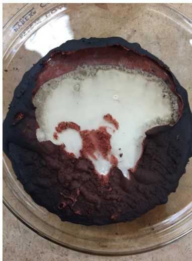
Figure 6. Visual observation of fixative “E” (white) layered with intumescent coating “FD” (red) on glass Petri dish after the intumescent coating was removed.
