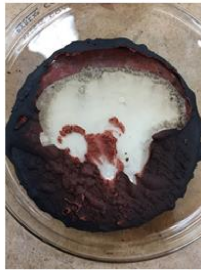
Fixative "E" with protective layer of selected intumescent coating "FD" after being subjected to 800° F for 15 minutes
