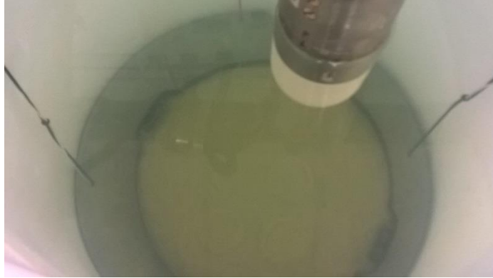
Figure 3. Photograph of the plastic lid filled with sand on a metal plate on the tank bottom.
