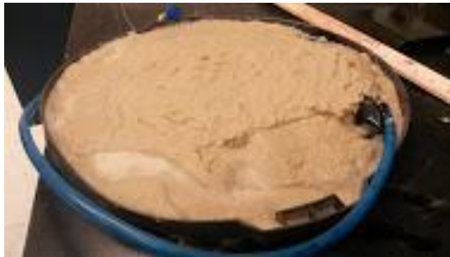
Figure 2. Photograph of air bladder mounted inside plastic lid with sand covering the bladder.
