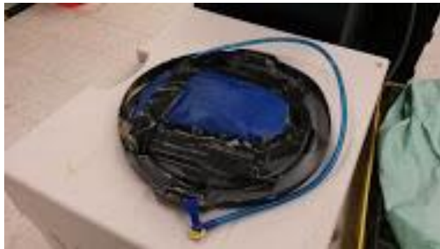
Figure 1. Photograph of the air bladder mounted with tape to the underside of a plastic lid.
