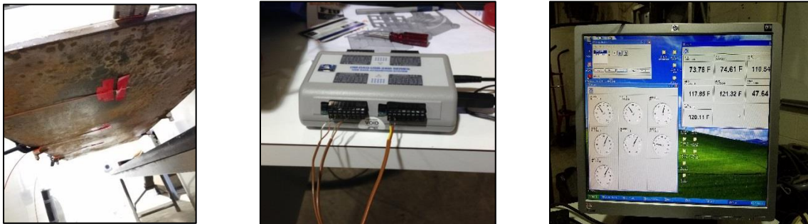
Figure 4. HSTs fixed under the plate (left), DAQ system with thermocouples (middle), DAQ dashboard (right).
