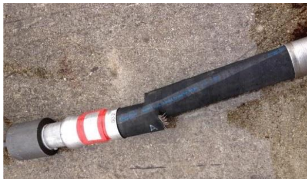
Figure 1. Ruptured HIHTL test specimen.
