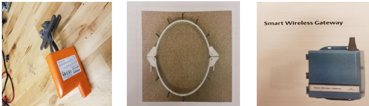
Figure 5. Permasense a) WT 210 series sensor b) Mechanical clamp c) Wireless Gateway (Emerson).
