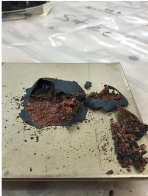
Figure 1. Example of FD adhesion to stainless steel substrate after exposure to 800° F.
