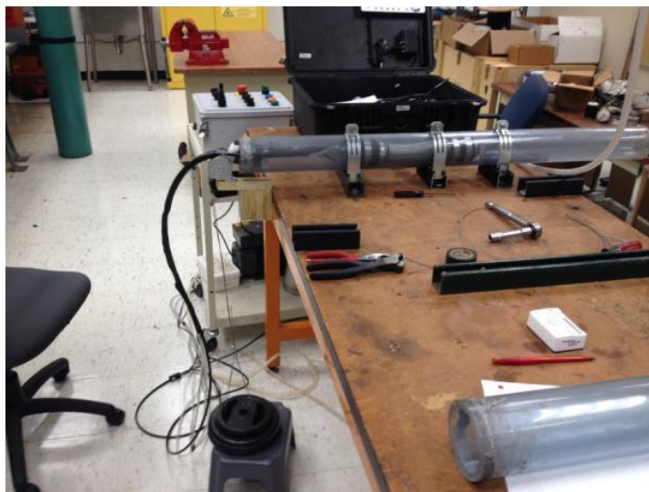
Figure 21. Testbed, pulley and weights set-up.
