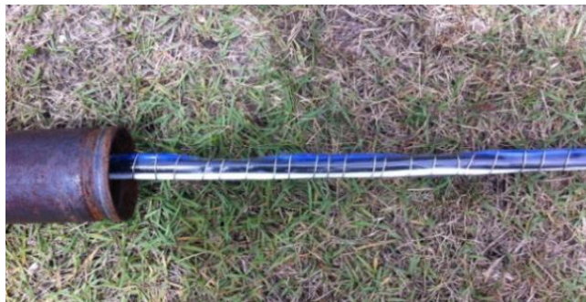
Figure 19. Tether with stainless steel coil.
