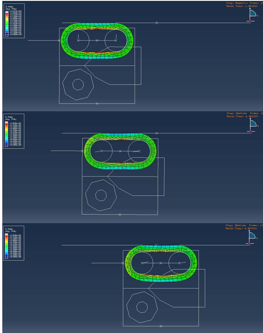
Figure 68. Inspection tool translating along tank bottom.
