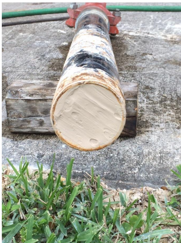
Figure 9. Plug blowout test.
