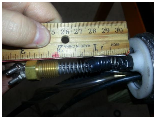
Figure 22. Rear washer and rear washer assembled to the crawler.
