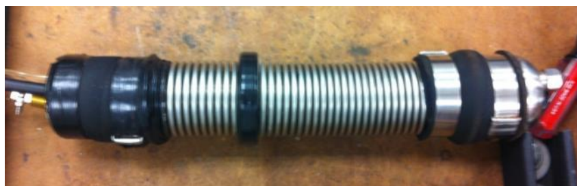
Figure 24. Ring prototyped, ring assembled on the crawler.
