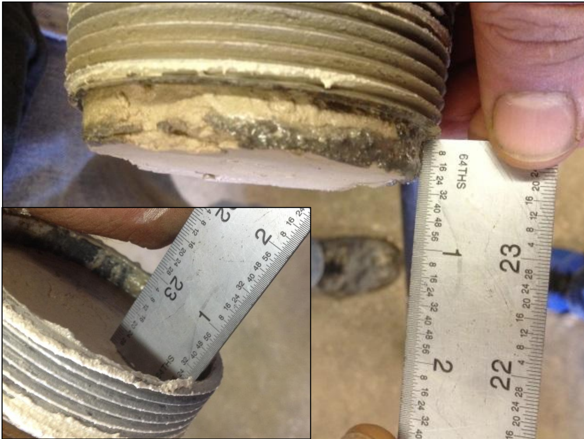
Figure 12. Kaolin-plaster plug after unplugging.
