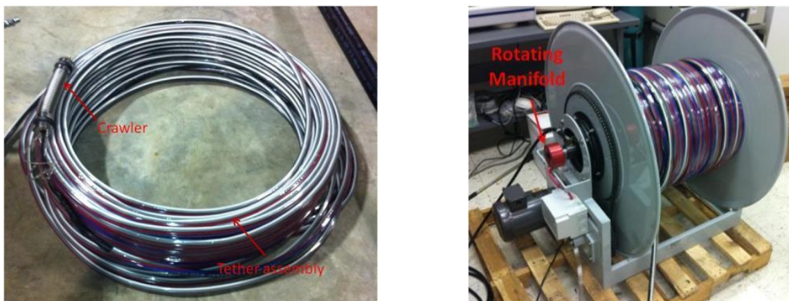
Figure 16. Tether attached to the crawler unit (left), tether-reel assembly (right).
