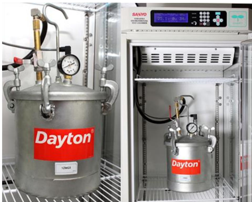
Figure 2. Isopiestic chamber to conduct solubility experiments connected to the acquisition system.
