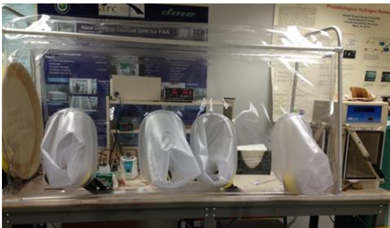
Figure 37 Anaerobic glove box
