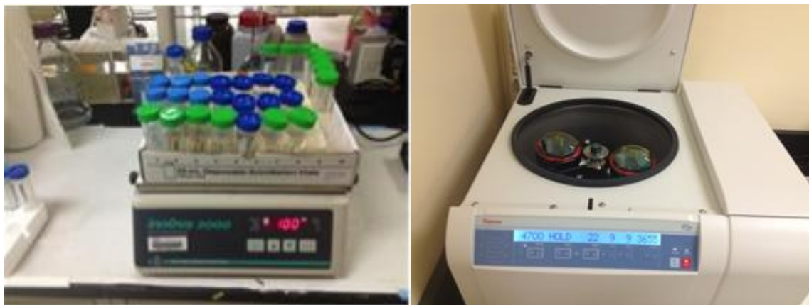
Figure 31. Conical tubes on the shaker at 100 RPM and centrifuge to separate supernatant
