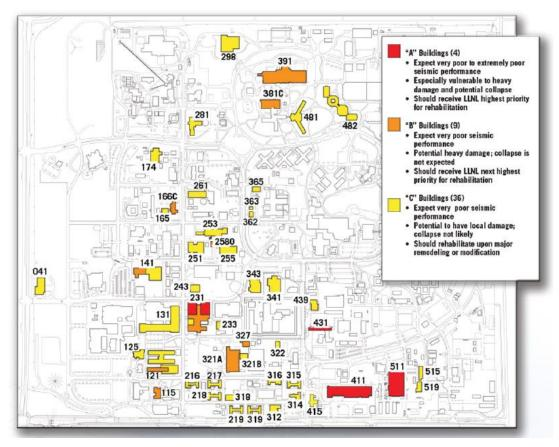
Figure 14. LLNL Site 200 buildings rated very poor in expected seismic performance. (Source: LLNL 2013)
