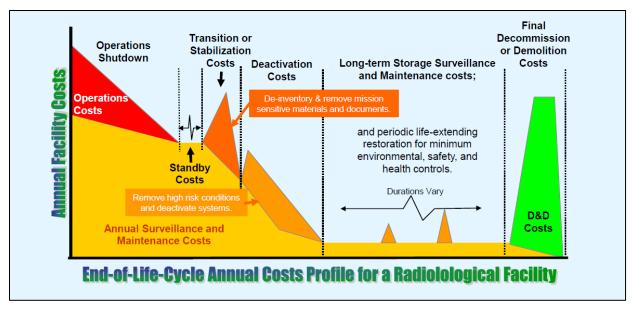
Figure 2. Typical End-of-Life Phases of a Nuclear Facility (Source: DOE 2011)
