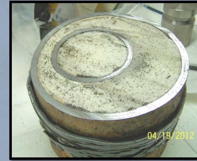
Figure 3. Photograph of the SN-278 Pipe-in-Pipe Section during sample unpacking.
