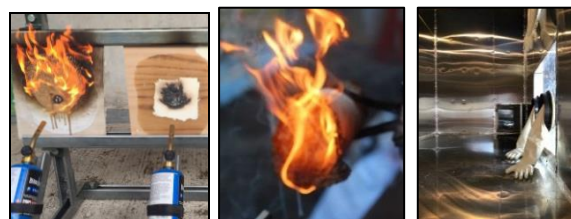
Testing fire resiliency of industry fixatives/IC/foams and hot cell test bed facility.
