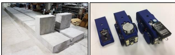
DST mockup facility and miniature rover with various sensors installed on top of the inspection tool.
