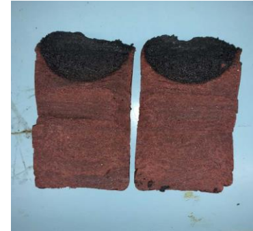
Intumescent Foam Sample cut in half Post Direct Flame Test
