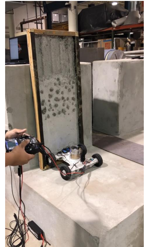
Testing of platform prototype 1 and 2 on concrete wall mock-up
