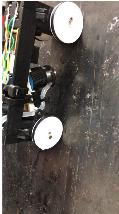
UT Rover obtaining thickness measurement
