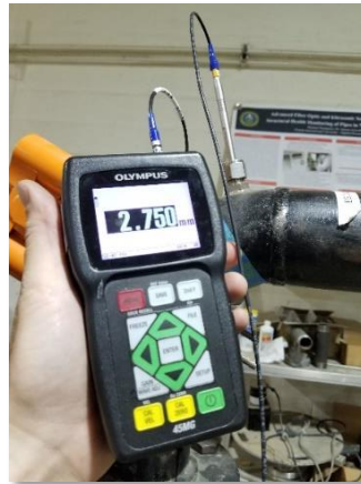
Thickness measurements using UT probe
