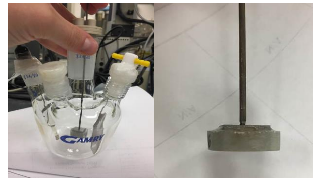
Experimental setup (left) and sample (right) for electrochemical measurements. Images provided by Mathew Asmussen, PNNL.
