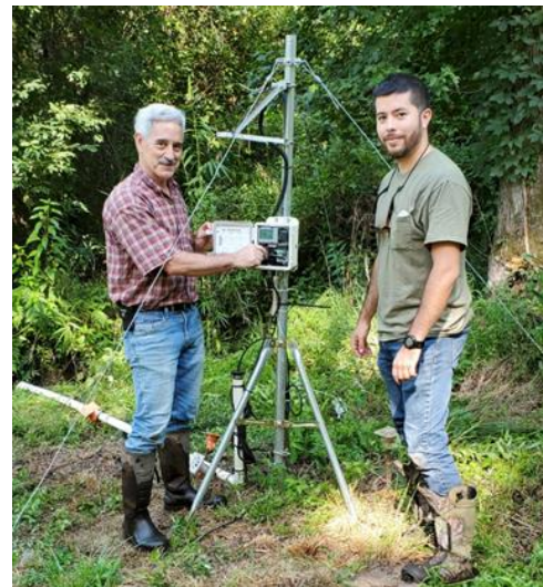
Left: DOE Fellow Juan Morales and Dr. Daniel Kaplan (SRNL) adding a turbidity sensor to the remote monitoring station in Tims Branch, SRS.
