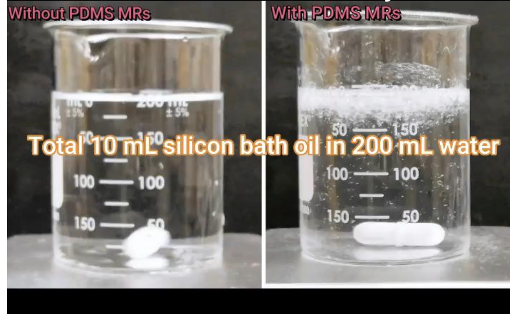
Test of PDMS-MRs adsorbability in water
