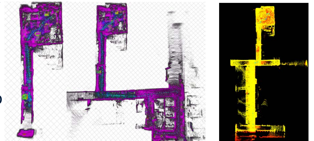
3D map constructed autonomously (left) and manually (middle and right) using mobile robot
