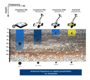
"The best antenna for a job is the one with the highest frequency that can still detect at the desired depth" -Geophysical Survey Systems (GSSI)
