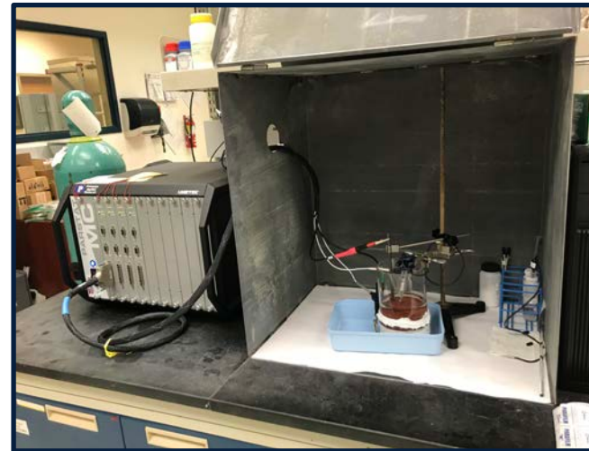
Potentiostat (left) and Faraday Cage (right) with test setup during impedance measurements
