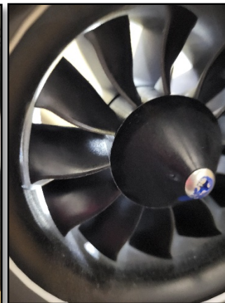
EDF unit with no significant blade damage
