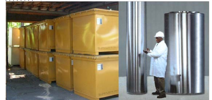
Containers for the storage of waste. Left: Carbon steel B-25 box for possible placement of cementitious waste forms, Right: Steel canister for LAW glass waste forms.
