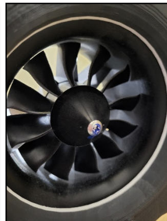
EDF unit with no significant blade damage
