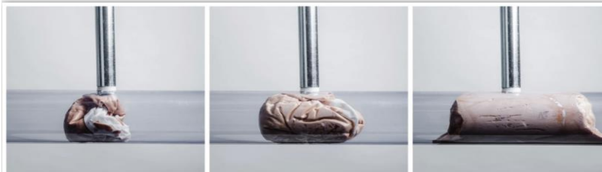
The FOAMBAG™ holds the resin foam in place as it expands. At full expansion some of the foam seeps through the semi-porous panels of the bag to form an adhesive seal with the pipe
