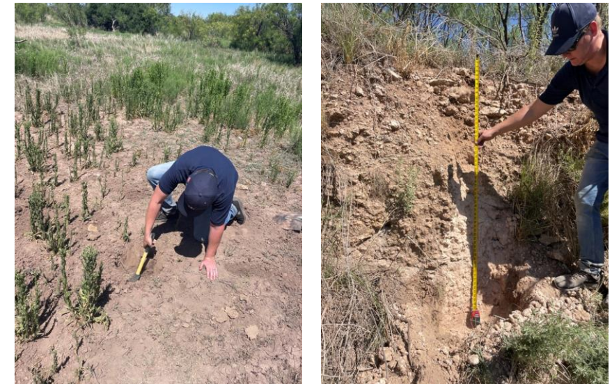
Collecting soil samples (left); soil variation near Location 1 (right).
