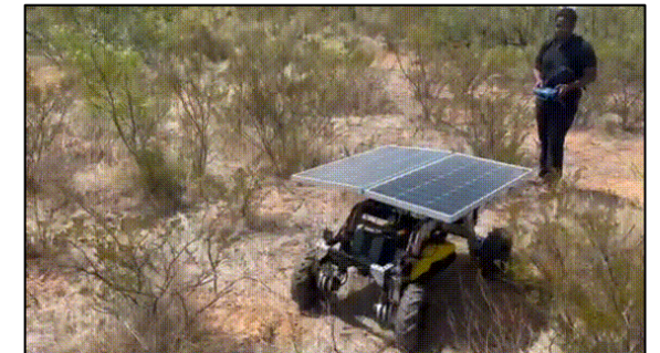
Using a GPR rover within Basin 6 (GPR rover developed in Project 5, Task 2).
