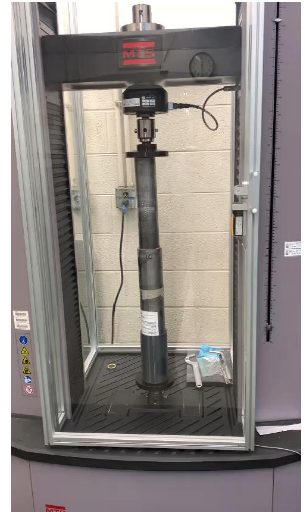
1 – Aluminum "Plunger" 2 – Pipe Foam Sample 3 – 3D printed (ABS) Bucket
