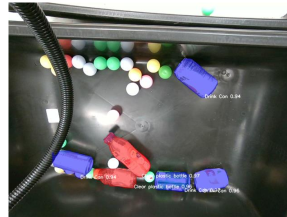
Figure 2: Live results from segmentation model looking inside the simulated waste bin
