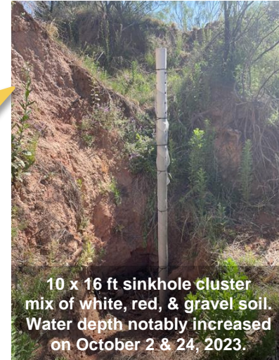
Location S1 (Sinkhole) with Transducer (T1)
