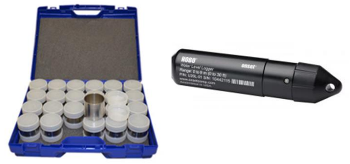
Left: Eijkelkamp soil sampling rings; Right: HOBO water level data logger.
