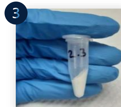
1) Stoichiometric Ratios used for HAp Synthesis. 2) Precipitate formed after 6 weeks. 3) Dried HAp
