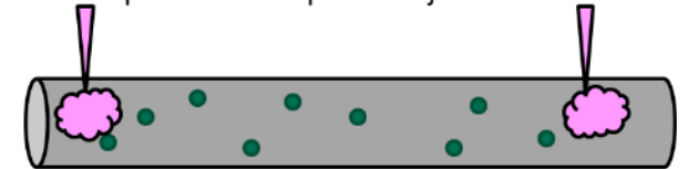
Use Hot Tap to Breach Pipe and Inject Fixative Foam
