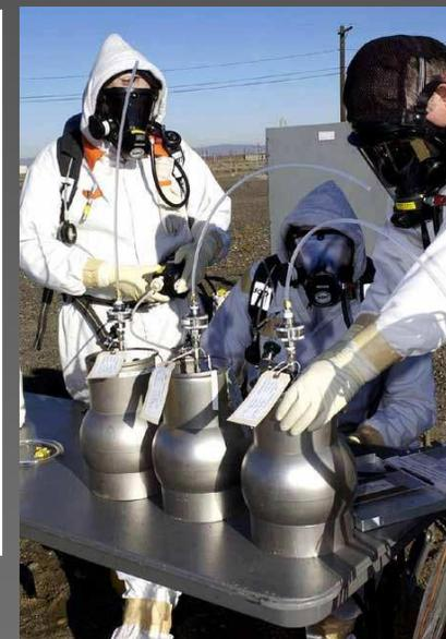
Workers replacing headspace vapor sampling with test ports in the tank outlet ventilation lines (source: RPP Facebook page, April 4, 2013)
