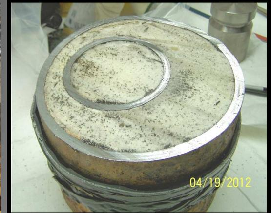
Photograph of the SN-278 Pipe-in-Pipe Section during sample unpacking.
