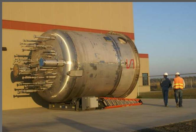
14-ft-diameter vessel to test PJMs
