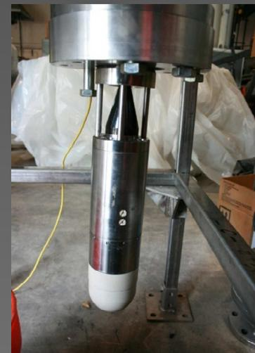
Right: sonar deployed through an 8-inch pipe similar to risers into million gallon HLW tanks
