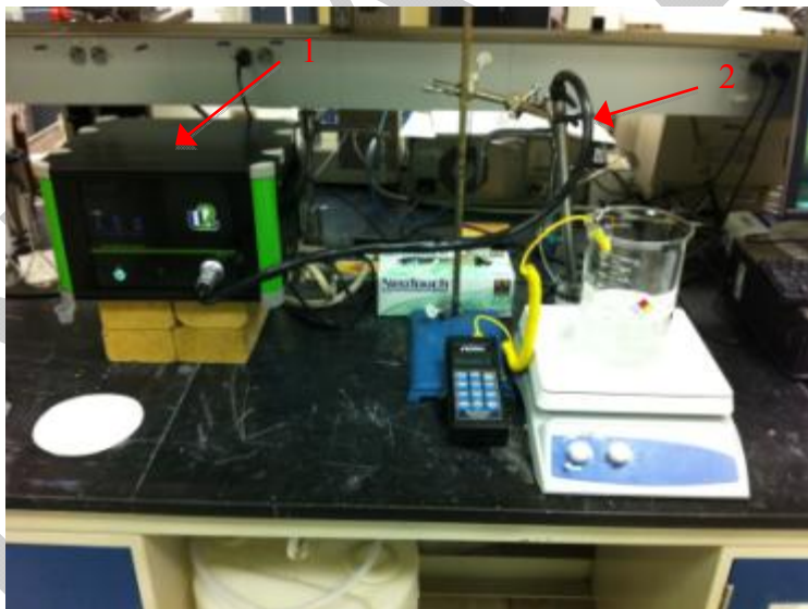
Figure 73. USS System installed in laboratory. The hardware components are shown: (1) controller, (2) probe.
