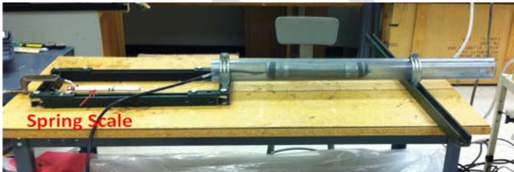
Figure 30. Testbed used to measure the pulling force.
