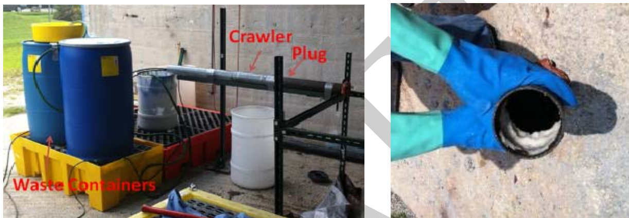
Figure 32. (a) Setup used to perform the sodium-aluminum-silicate unplugging test, (b) pipe after unplugging operation.
