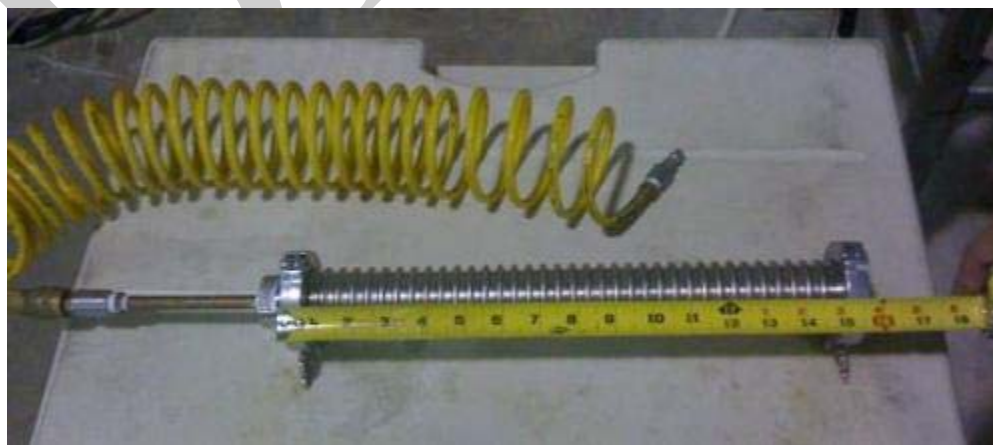
Figure 22. Burst pressure test on hydro-formed bellow.
