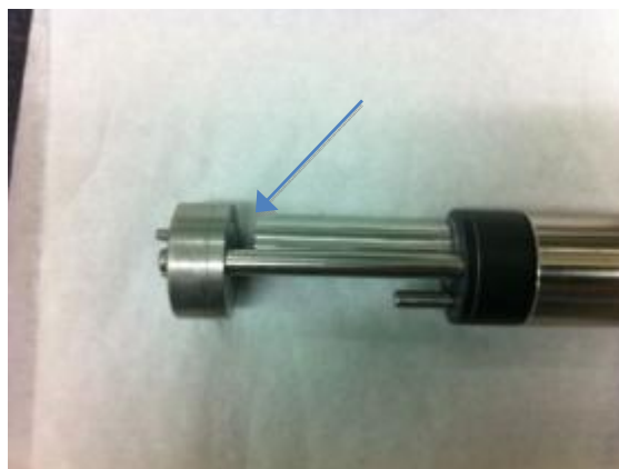
Figure 75. 36 mm spacers reduced the propagation path to 3.83 mm, allowing for higher solids concentration in the media under test.
