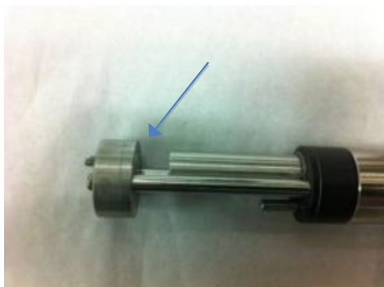
Figure 74. 40 mm spacers provided a 7.83 mm propagation path for the ultrasonic pulse.
