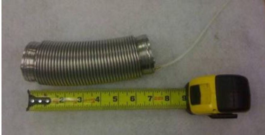
Figure 23. Double walled bellow assembly contracted due to vacuum pressure.
