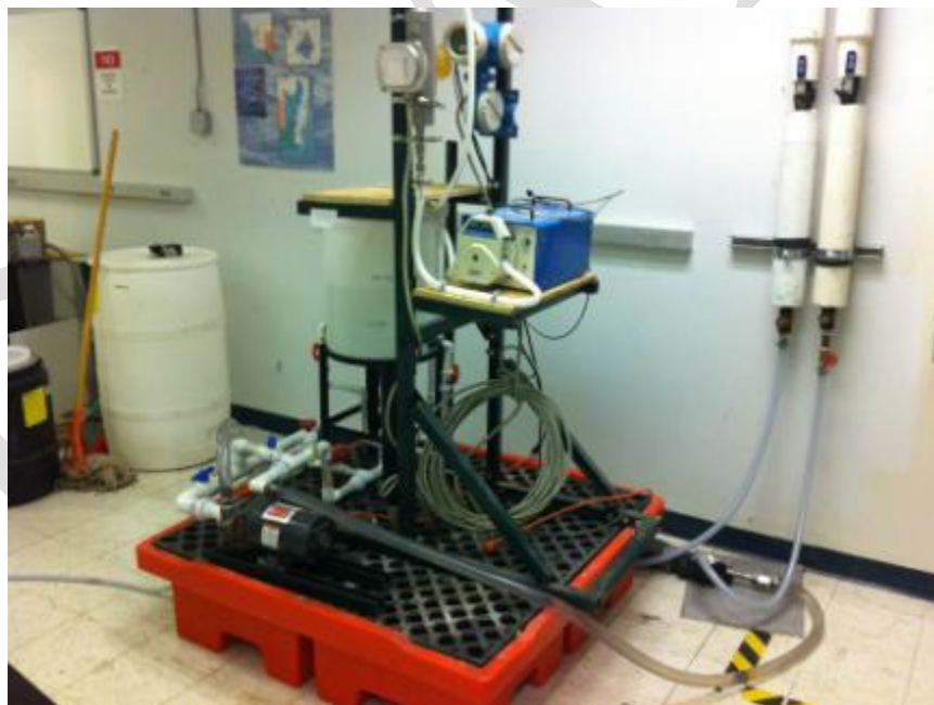
Figure 71. Sampling loop at FIU. The sampling pump and Coriolis meter are visible in the center and top of the image.
