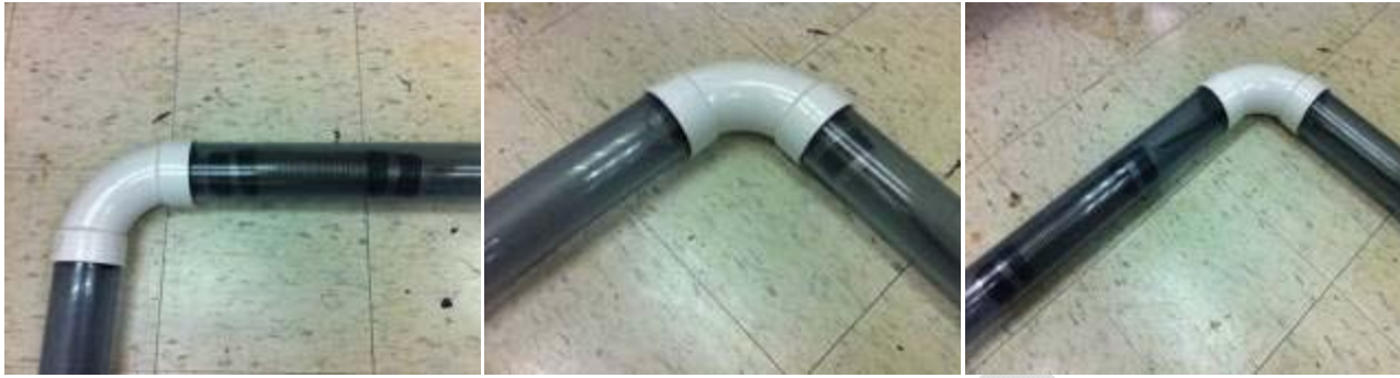
Figure 29. Sequence of crawler turning through an 90° elbow.
