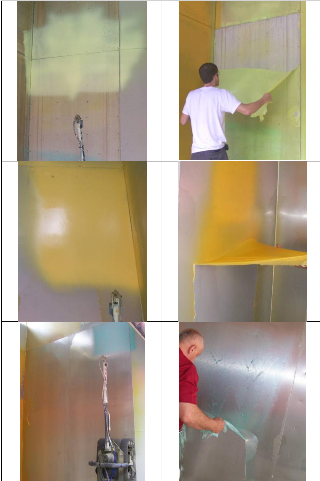
Figure 6. Wet coatings being applied remotely by sprayer (left) and dry coatings being stripped manually (right): CC Strip on concrete panel (top), ALARA 1146 on steel panel (middle), and DeconGel on steel panel (bottom).
