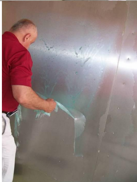
Stripping DeconGel from steel panel. Coating applied prior to demonstration.
