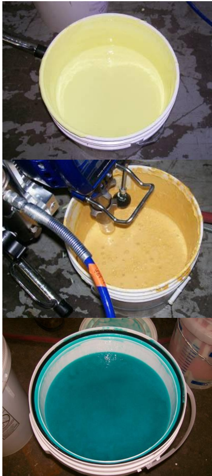
Strippable coating products (from top): CC Strip, ALARA 1146, DeconGel
