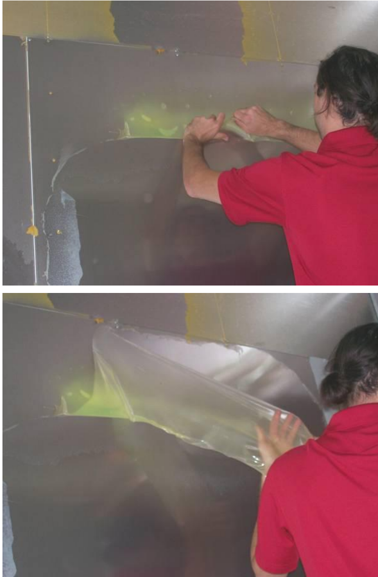
Stripping CC Strip from steel panel. Coating applied prior to demonstration.
