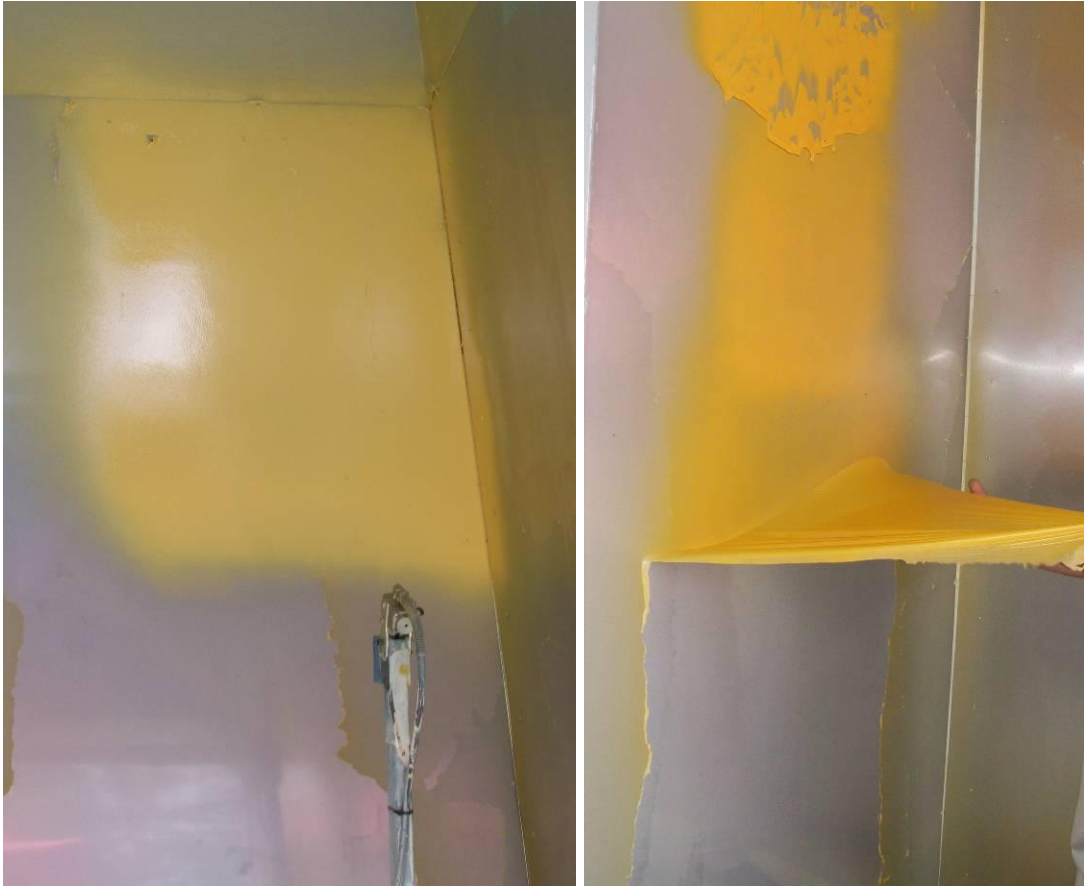
Figure 5. ALARA 1146 being sprayed onto a steel panel (left) and dry ALARA 1146 being removed from a steel panel (right)
