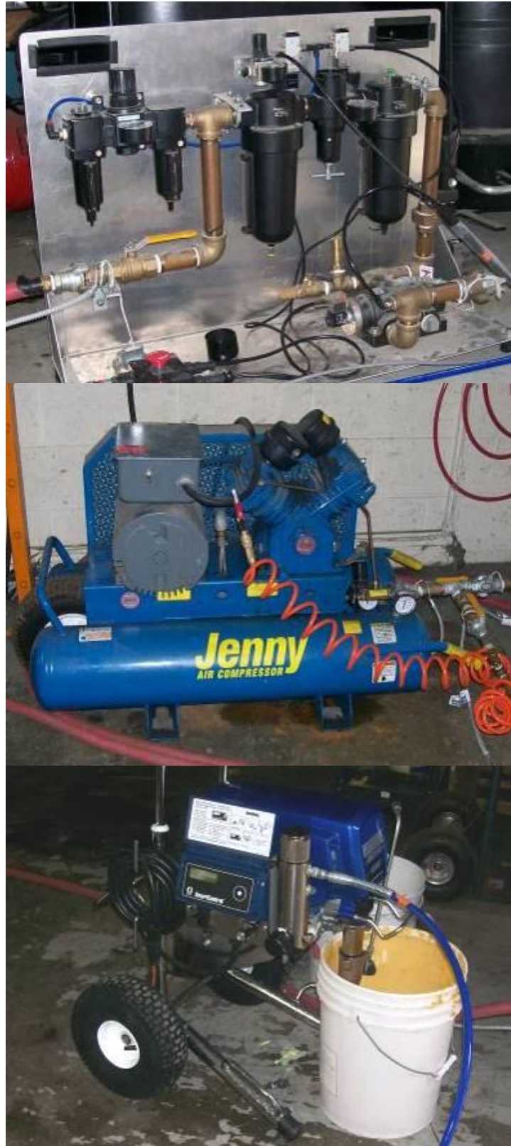
Equipment used (from top): junction box, Jenny air compressor, Graco spray unit
