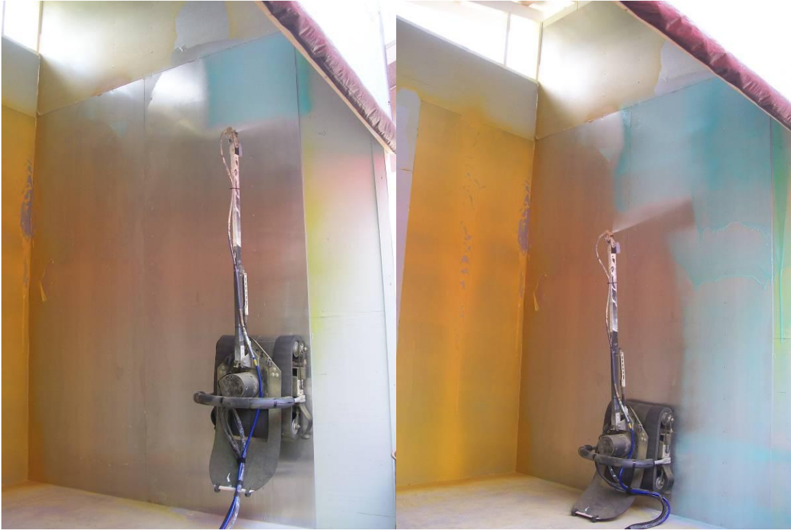
Spraying DeconGel on steel panel.
