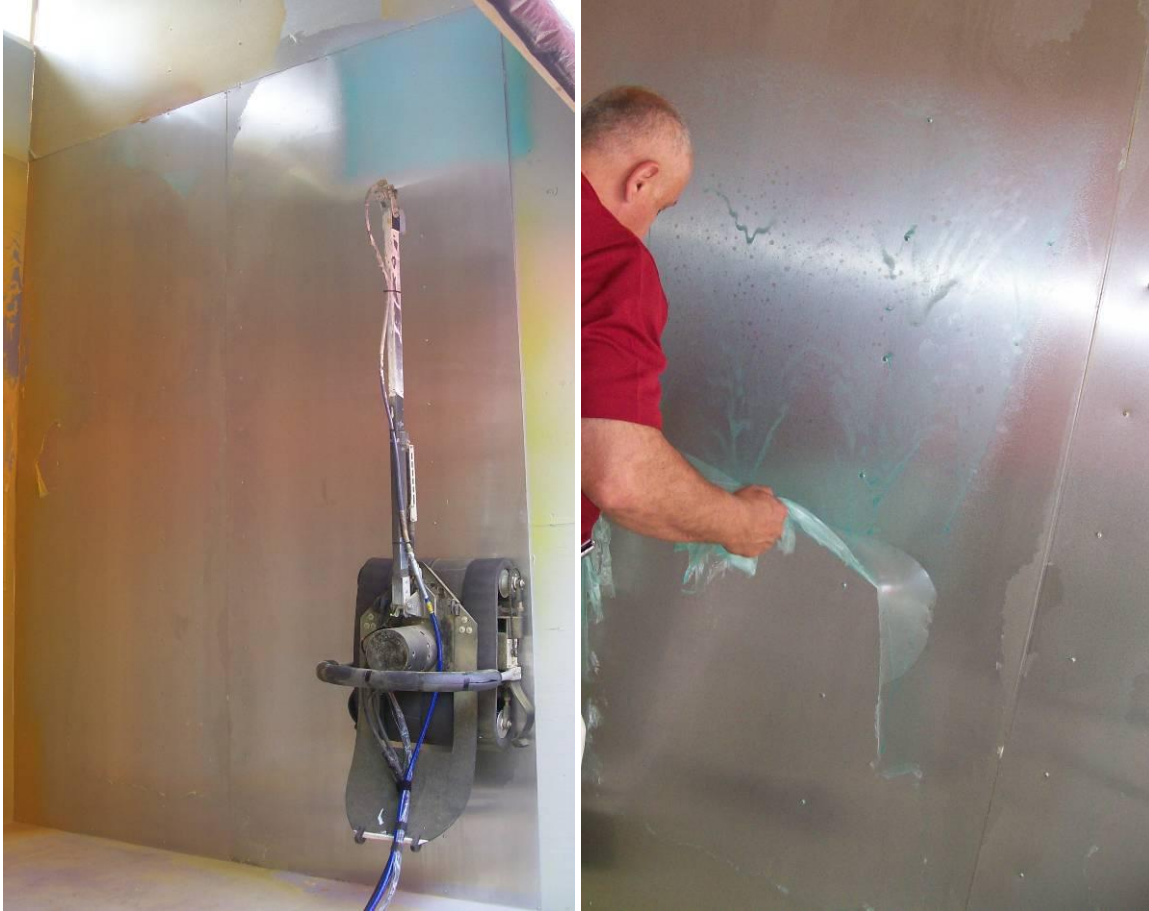
Figure 6. DeconGel being sprayed onto a steel panel (left) and dry DeconGel being removed from a steel panel (right)
