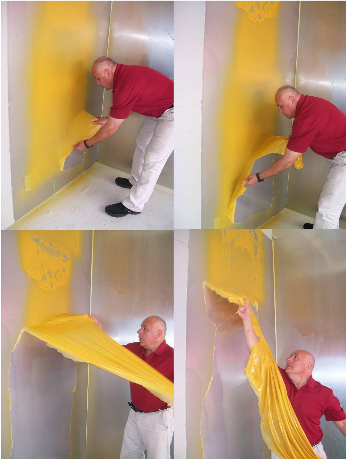
Stripping ALARA 1146 from steel panel. Coating applied prior to demonstration.
