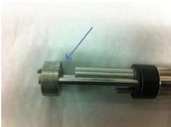
**Figure 52. 40 mm spacers provided a 7.83 mm propagation path for the ultrasonic pulse.**
