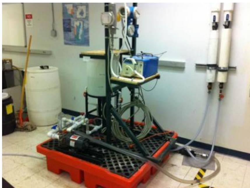
**Figure 49. Sampling loop at FIU. The sampling pump and Coriolis meter are visible in the center and top of the image.**
