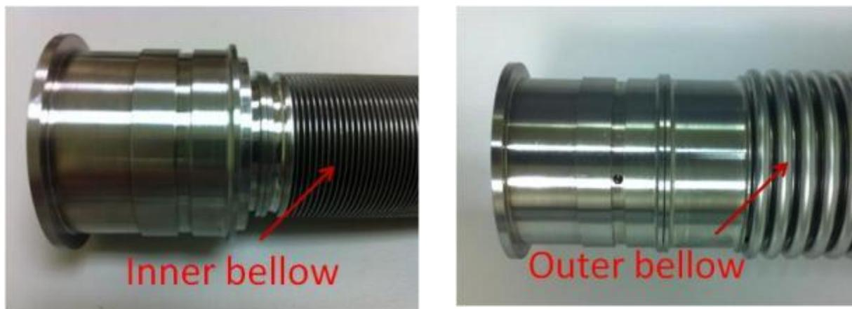
**Figure 24. A) Inner bellow and rim, B) Outer bellow and rim.**
