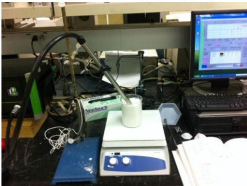
**Figure 50. Benchtop test setup. Preliminary solids loading tests and troubleshooting were performed in this setup.**
