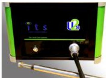
Figure 45. USS System Control Module and In-tank probe
