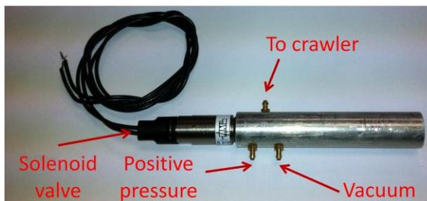
**Figure 32. Solenoid/manifold prototype.**
