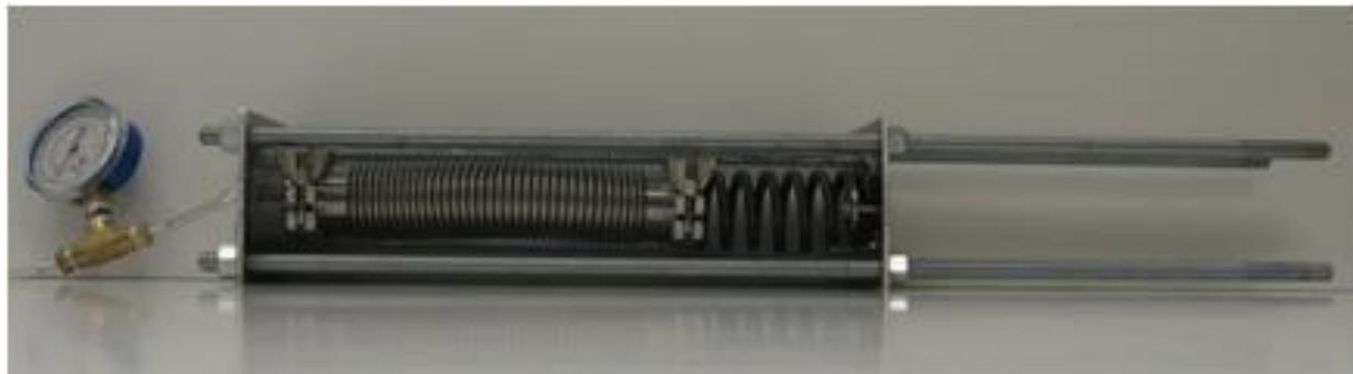
**Figure 27. Setup used for bellow response tests.**
