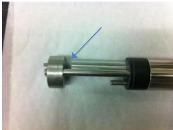
**Figure 53. 36 mm spacers reduced the propagation path to 3.83 mm, allowing for higher solids concentration in the media under test.**
