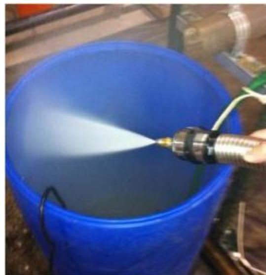
**Figure 31. A) Rotating nozzle B) 15° angle degree nozzle.**
