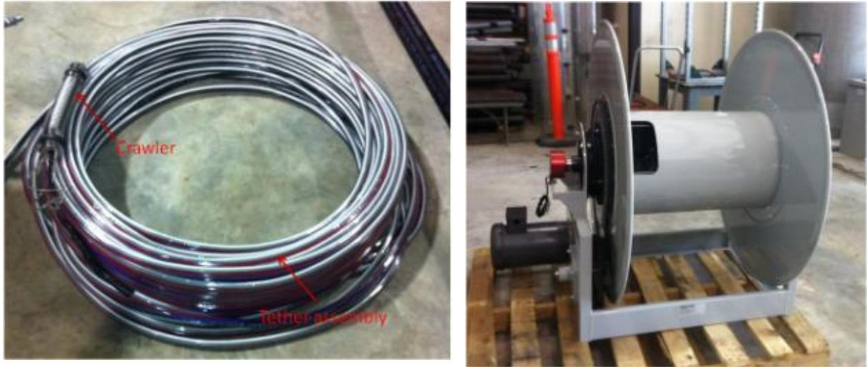
**Figure 25. A) Tether attached to the crawler unit, B) Reel system.**
