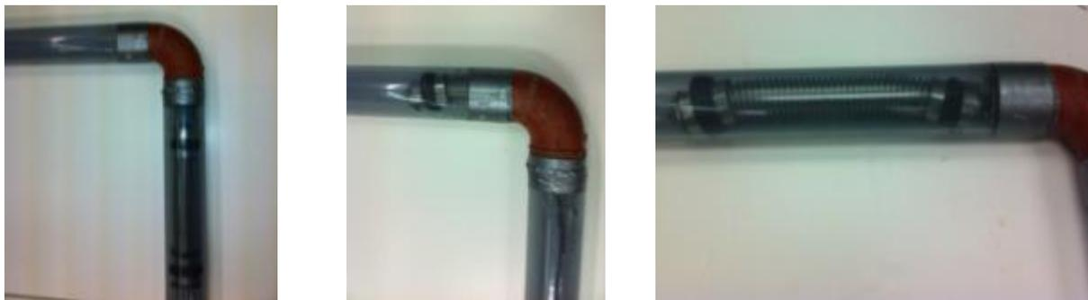
**Figure 29. Sequence of crawler turning through a 90° elbow.**
