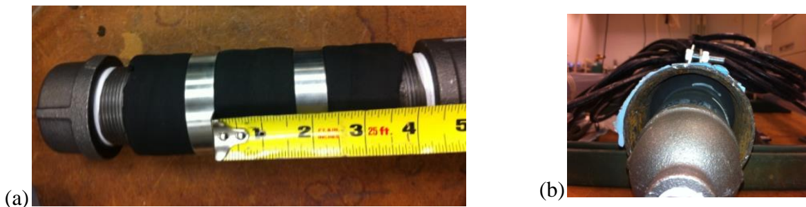
Figure 30. Experimental fixture and experimental fixture inside pipeline section.
