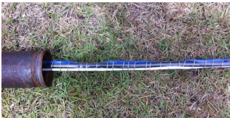
Figure 27. Tether with stainless steel coil.
