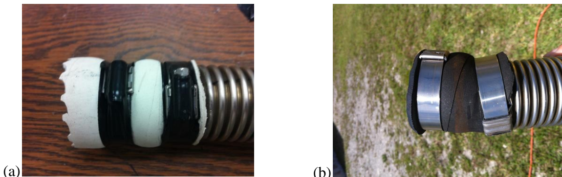
Figure 29. (a)Back rim with 0.125 in thick flexible gum, (b)failure due to insufficient clamping force.
