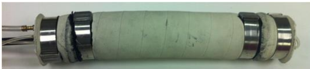
Figure 21. Crawler with a 0.125 in thick sleeve.
