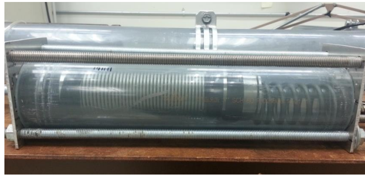
Figure 23. Fixture used to determine the crawler unit force.
