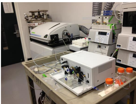
Figure 21. Coupling of a Flow Injection System (FIAS 400) to ICP-MS for analyzing mercury isotopes.
