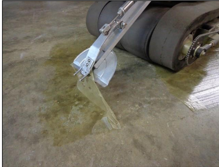
Figure 5. ICM remote platform with a gripper/scrapper tool to remove strippable coatings.
