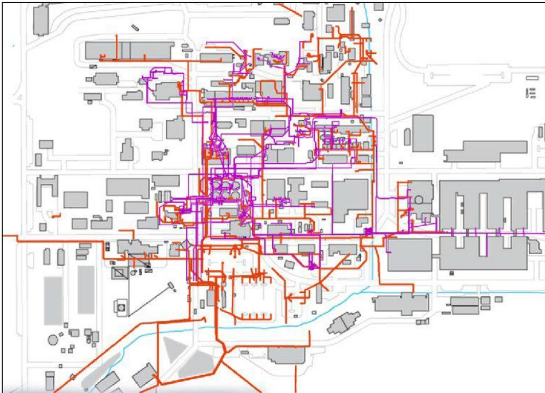
**Figure 26. Underground pipelines at ORNL: liquid low-level waste lines in magenta and process waste pipelines in orange (Source: Schneider 2012).**
