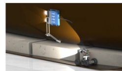
A magnetic crawler and 4-wheeled robot inspecting the annulus space and refractory air slots
