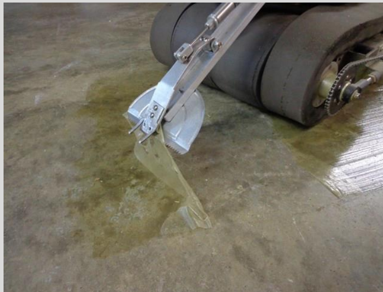
Figure 4-3. ICM remote platform with a gripper/scraper tool to remove strippable coatings.
