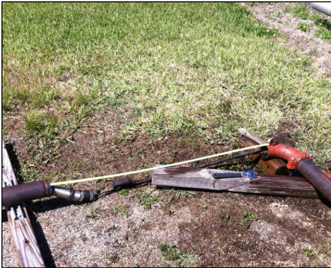
Figure 1-5. Largest distance achieved after elbow, failure of the pneumatic lines at the valves.
