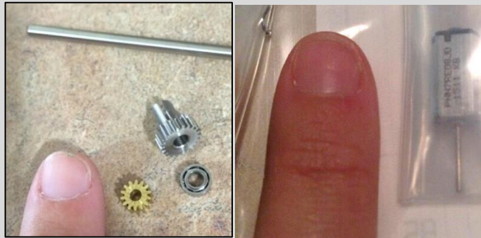
Figure 1-43. Components: gears, bearing, shaft, and motor.
