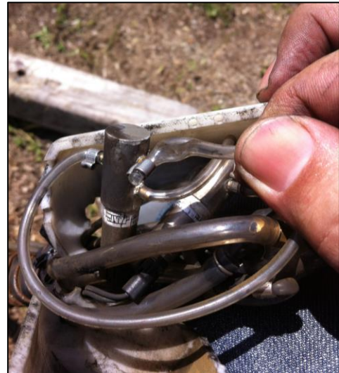
Figure 1-5. Largest distance achieved after elbow, failure of the pneumatic lines at the valves.
