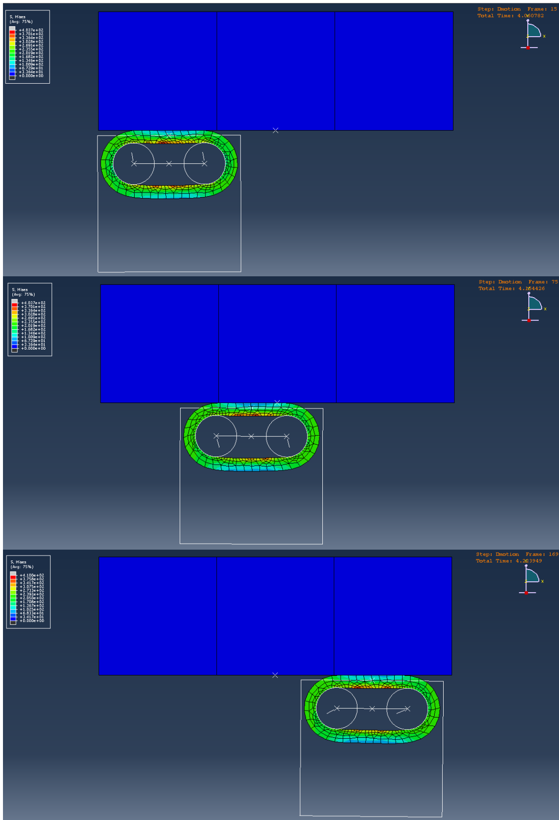
Figure 1-34. Inspection tool translating under torque load applied at real wheel.
