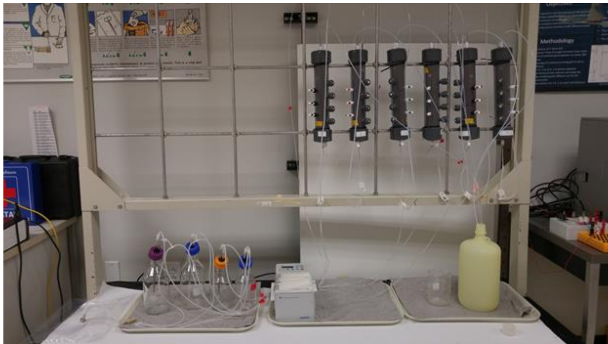
Figure 2-22. Experimental set up with six columns. The set up allows for the collection of SIP measurements and enables correlation of the data with changes in the columns' porewater geochemical parameters.
