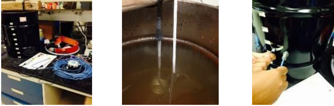
Figure 1-47. a) Bench scale test set up, b) immersion coil, and c) thermocouple and Raytek sensor head.
