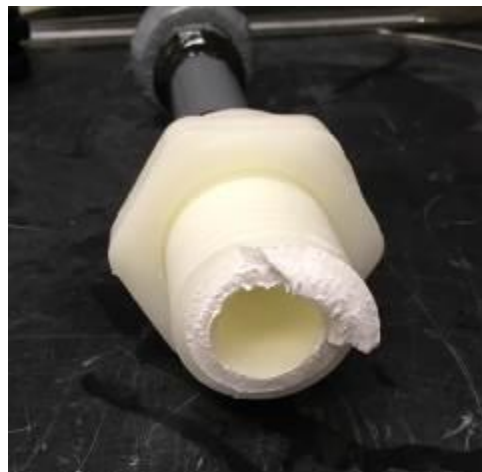
Figure 1-58. Cracked 3/4" polyethylene bulkhead fitting.
