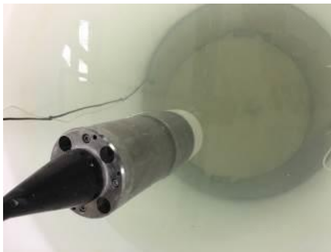
Figure 1-13. Sonar in the test tank and the target circular disc of sand.
