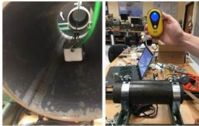
Figure 1-43. (a) Deployment inside pipe, (b) Magnetic force measurement set-up.
