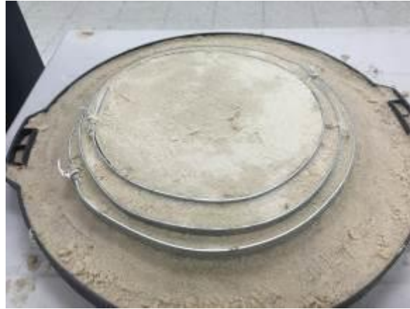
Figure 1-23. Test object with circles of sand of varying heights and diameters measured to mm resolution.
