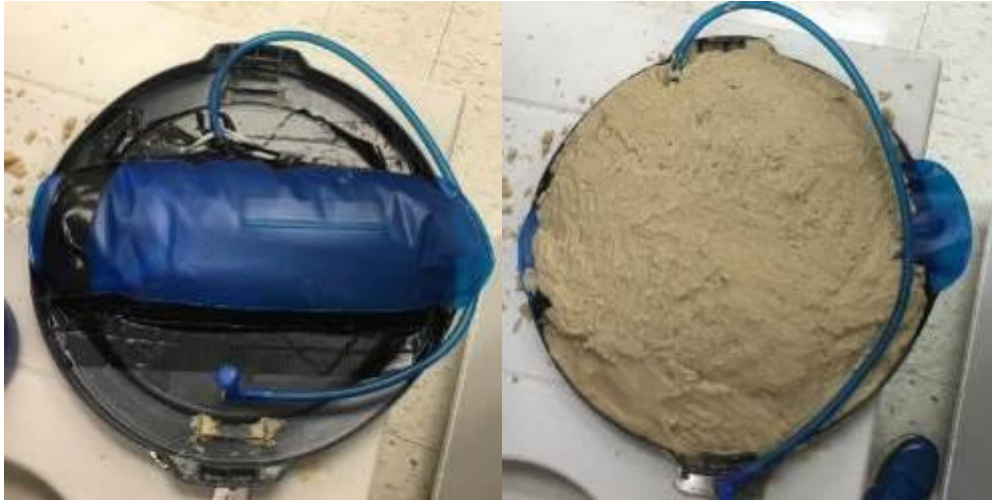
Figure 1-15. Photographs of air bladder mounted inside plastic lid and with sand added covering the bladder.
