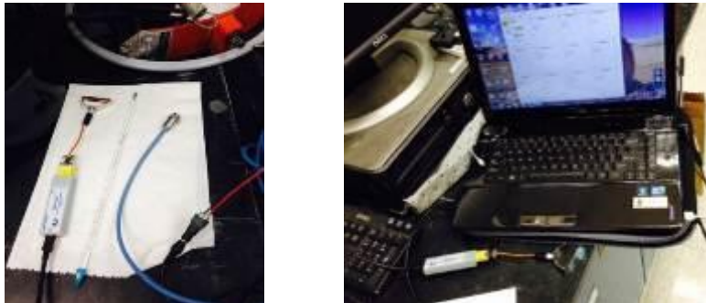
Figure 1-48. a) Equipment for temperature readings, b) data acquisition using the UTC-USB connector.
