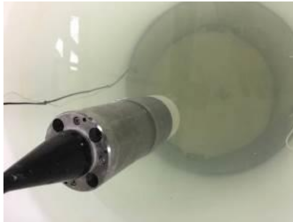
Figure 1-16. Photograph of sonar in the test tank with metal plate and plastic lid, bladder and sand.
