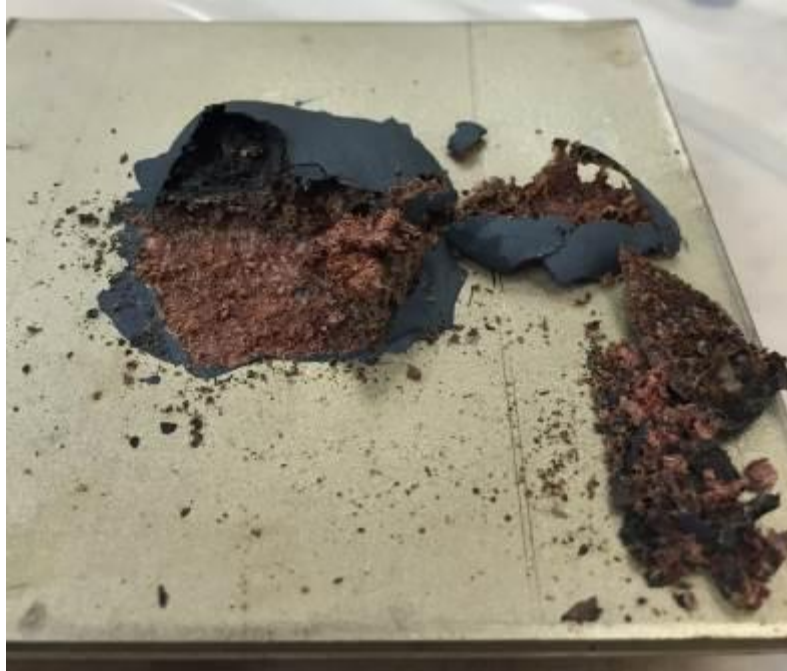
Figure 3-3. Fire Dam intumescent coating after exposure to 800° F.
