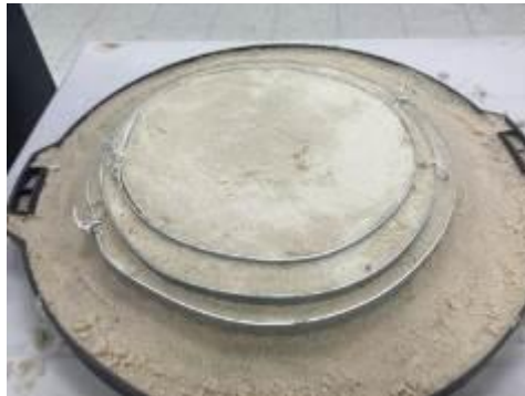
Figure 1-19. Test object with circles of sand of varying heights and diameters measured to mm resolution.
