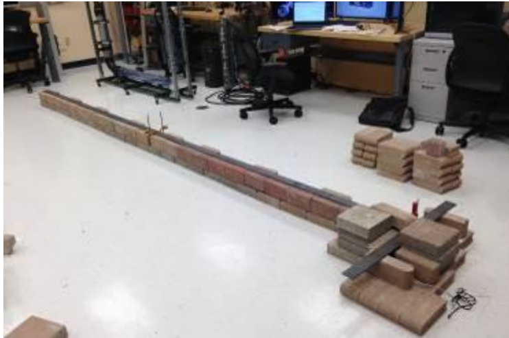
Figure 1-44. Laboratory scale test bed created for determining the pull force created by tether.
