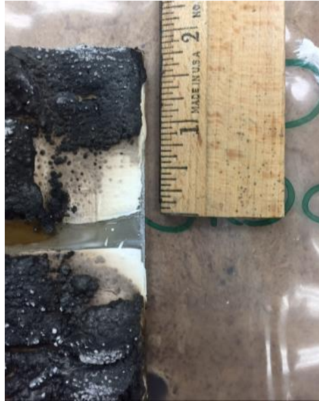
Figure 3-7. Charred intumescent coating provided thermal protection to bordering fixative.
