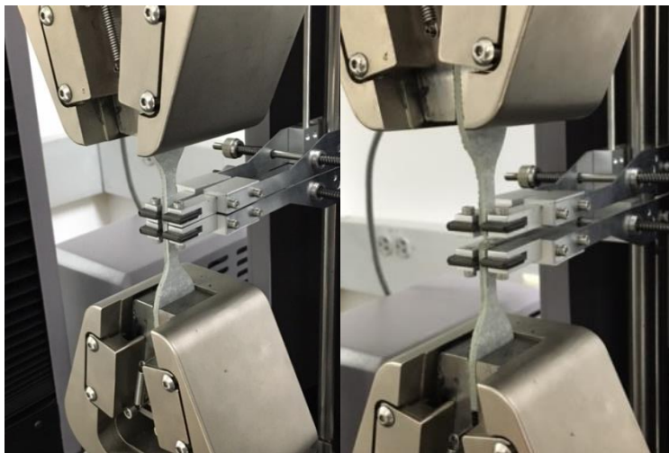
Figure 1-44. Garlock coupon testing.
