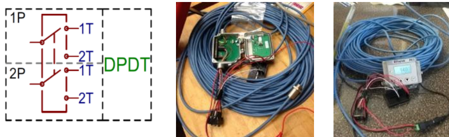
Figure 1-32. Switch circuit symbol (left), circuit assembly – open (center), circuit assembly – closed (right).
