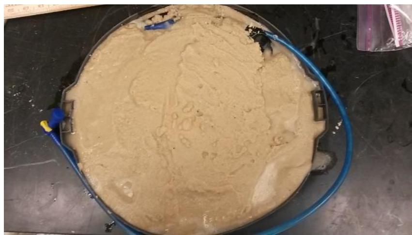
Figure 1-9. Same air bladder covered with paver sand to create object to be imaged by the 3D sonar.
