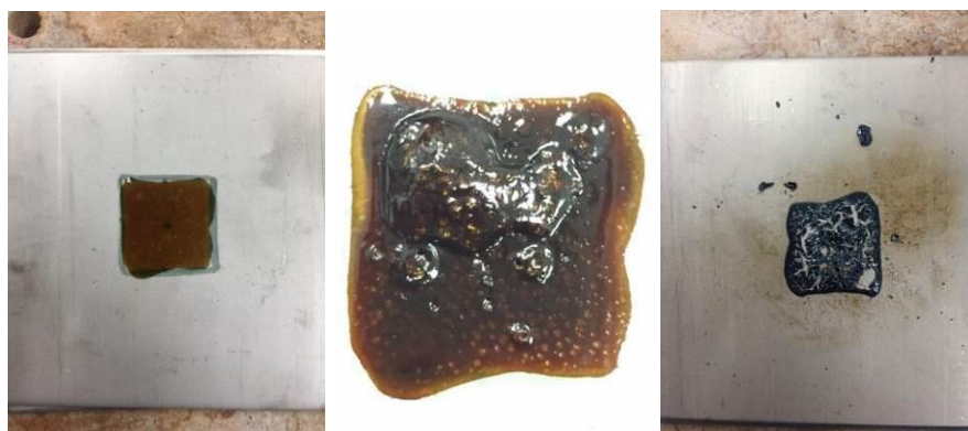
Figure 3-2. Fixative A, from left: after exposure to 400°F, 600°F, and 800°F.
