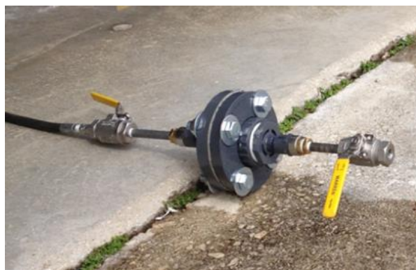
Figure 1-48. Gasket baseline pressure test rig.
