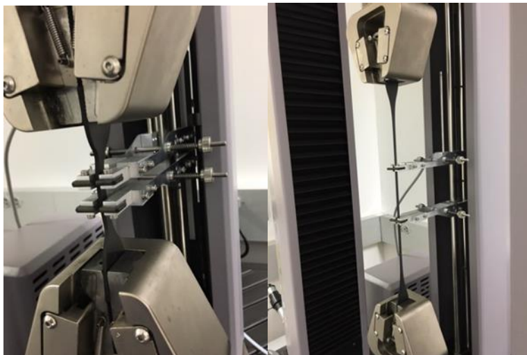
Figure 1-42. EPDM coupon testing.
