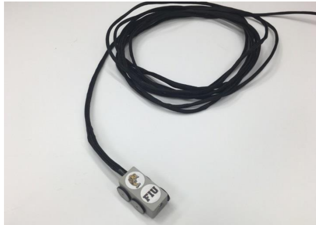
Figure 1-14. Prototype of completed design for the miniature rover inspection tool.
