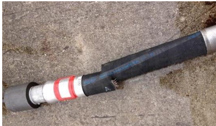
Figure 1-46. Ruptured HIHTL test specimen.
