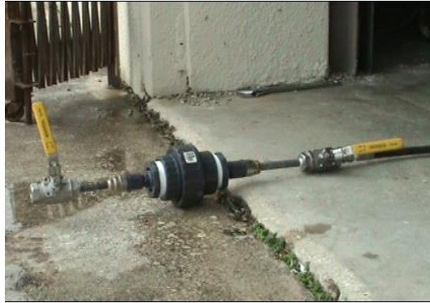
Figure 1-47. O-ring pressure test rig.
