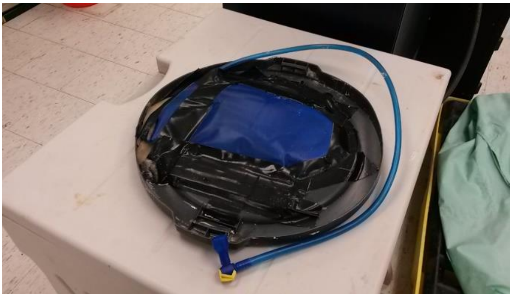
Figure 1-8. Air bladder with metal weights underneath taped to a plastic lid.
