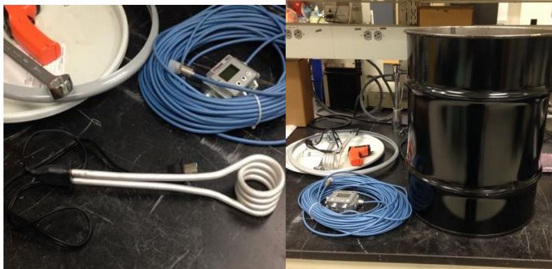
Figure 1-31. a) immersion coil and b) carbon steel drum.
