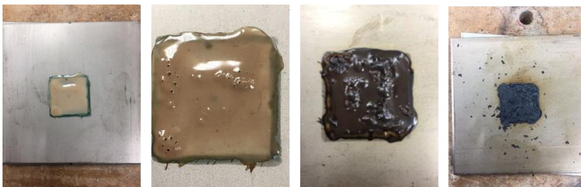
Figure 3-3. Fixative B, from left: after exposure to 200°F, 400°F, 600°F, and 800°F.
